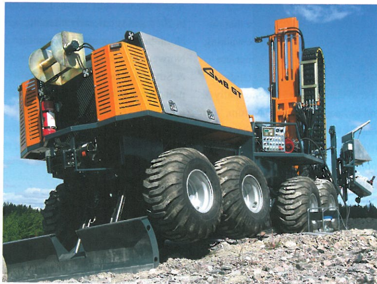
The GM8 body driven, rubber-wheeled drilling rig has been specifically designed for use in the urban environment
